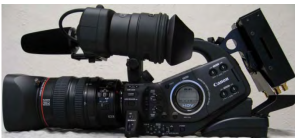
Flash XDR Mounted to Back of Camcorder
